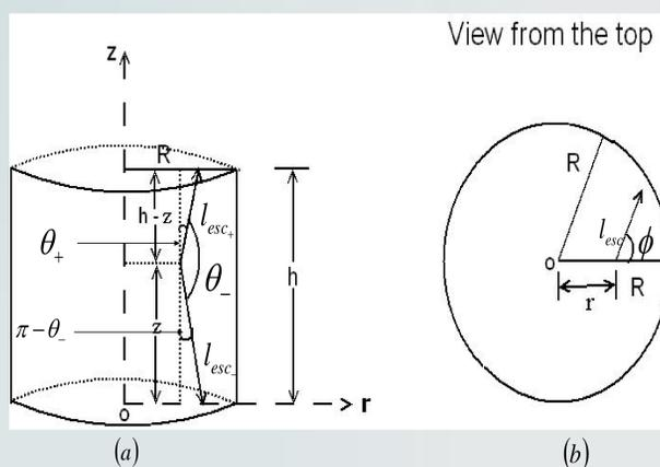
**Fig. 2:** (a) Depiction of the three possible directions (forward, backward & sideways) of escape for photons from a cylinder.  $l_{esc+}$  is the escape length for the forward direction making an angle with the axis of the jet (z-axis), &  $l_{esc-}$  is that for the backward direction.
